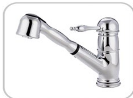
KFC-024-0062 Pull-Out Kitchen Faucet (Over All Height)220 mm / (Spout Height)166.5 mm / (Spout Length)232.5mm Brass Alloy / Plated Chrome
