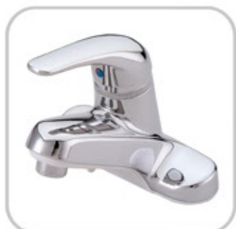
KFC-026-0047 4 in. Single Handle Lavatory Faucet Over All Height : 125.8 mm / Spout Height Deck : 52.1 mm / Spout Length : 107.4 mm Zinc Handle and Housing / Plastic Bottom / Lead Free Brass Water Way Plated Chrome
